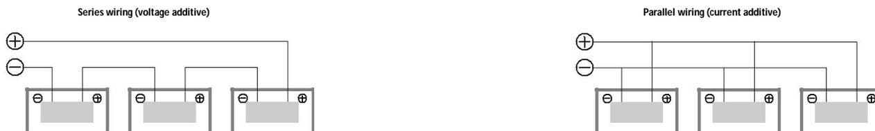
Figure 5: Electrical diagrams of series and parallel wiring
